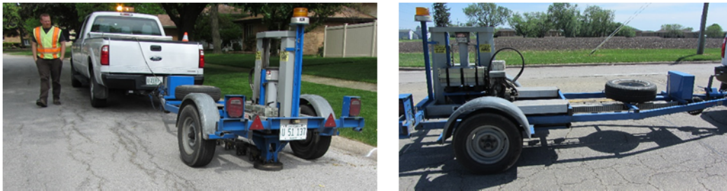
Figure 1. Conducting FWD tests in selected local road pavement sections in Illinois.
